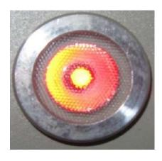
When the status indicator lamp shows green, it indicates that the program is running status; when the status indicator lamp shows red, it indicates that the program is setting status. (tips: if the lamp changes from green to red when the machine is in running status, press F5 into the running status again).
