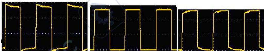
Figure 3-7 Displayed Waveforms of the Probe Compensation
