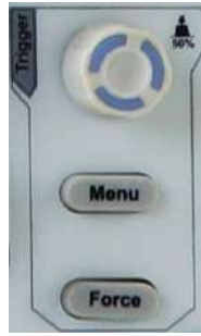
Figure 3- 13 Trigger Control Zone
