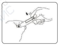
(2). Please take out the upper cover of test pencil according to the direction as shown in the picture, replace the battery. (see the following picture)
