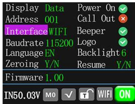
★★ Note: after the communication interface is set to WiFi, wz6008 needs to be reset After restart, the interface of wz6008 is as follows:
