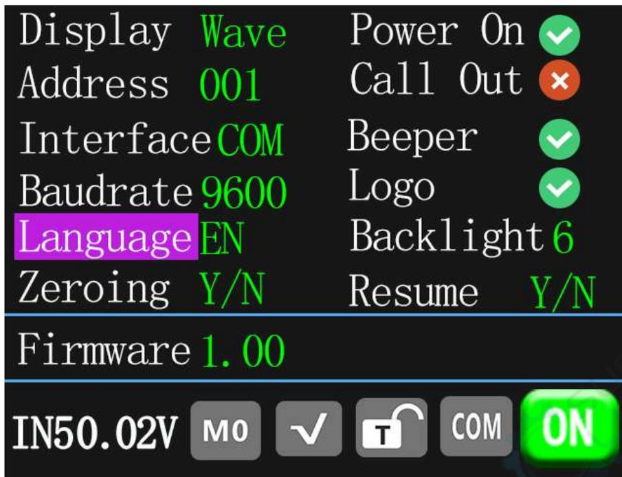
Press the direction key to select the setting option. The red reverse display is the selected position. Rotate the encoding potentiometer to change the setting.
