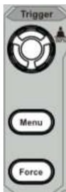
Figure 3-12 Trigger Control Zone
