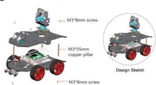
The two-layer structure assembly is completed, and this structure can realize functions: remote control mode, track mode, obstacle avoidance mode, seven-color inspection,
