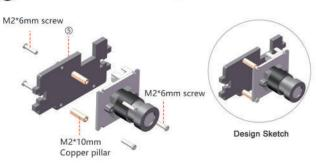
07 Assemble rotating arm and fixing board
