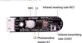
Infrared obstacle avoidance & light seeking module
