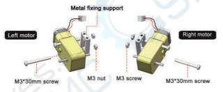
Screw+fixing support+motor (Two motors on the each side, the fixing bracket is mounted on the side of the motor wiring, the screw holes is facing upwards.) M3\*8mm screw
