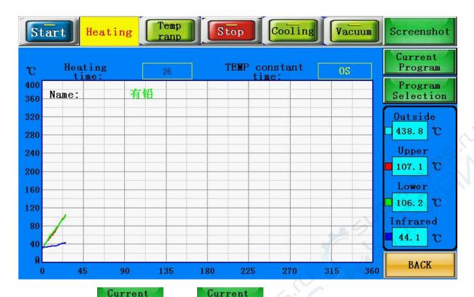
15)Current curve **Program**: Click **Program** to get in the current curve frames, the following picture shows the working temperature parameters after starting heating. They are target temperature, constant temperature time, and the speed of heating (the speed of heating with °C/SEC calculation).
