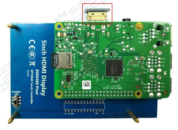
2) Connect The LCD and Raspberry Pi with the HDMI adapter.
