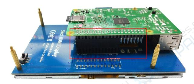
1) Connect The LCD 13\*2 Pin socket to Raspberry Pi as the Picture show above.
