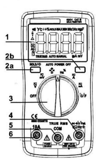
(1) LCD Display Screen: Measuring values and unit will be displayed on the screen.
