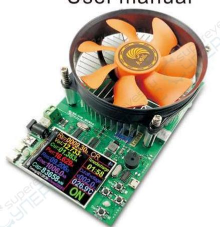
This product is used to inspect and test the capacity of various batteries , discharge and aging various power adapters, USB chargers, various mobile power and other power supply equipment
