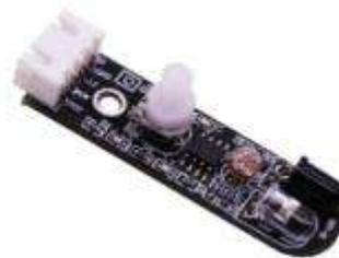
1-2 Infrared obstacle avoidance module
