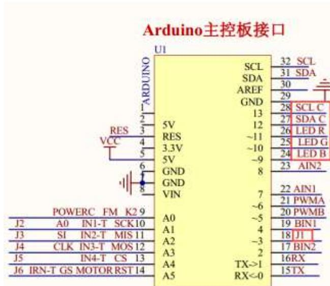
4-1 Arduino UNO interface circuit diagram
