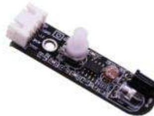
1-2 Infrared obstacle avoidance module
