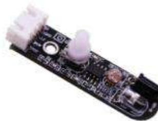
1-2 Infrared obstacle avoidance module
