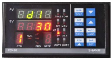
5) r2means the 2<sup>nd</sup> temperature rate,we set3.00, press can decrease and increase and increase and increase and increase and increase the figure, after finishing, press set to continue.
