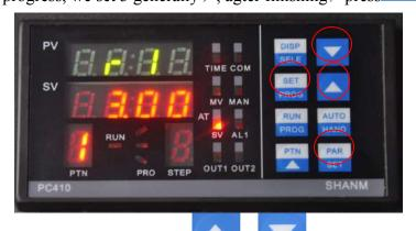
3) L1means the first seted temoweature, press can increase and decrease the fgure, we set165, press set to continue.
