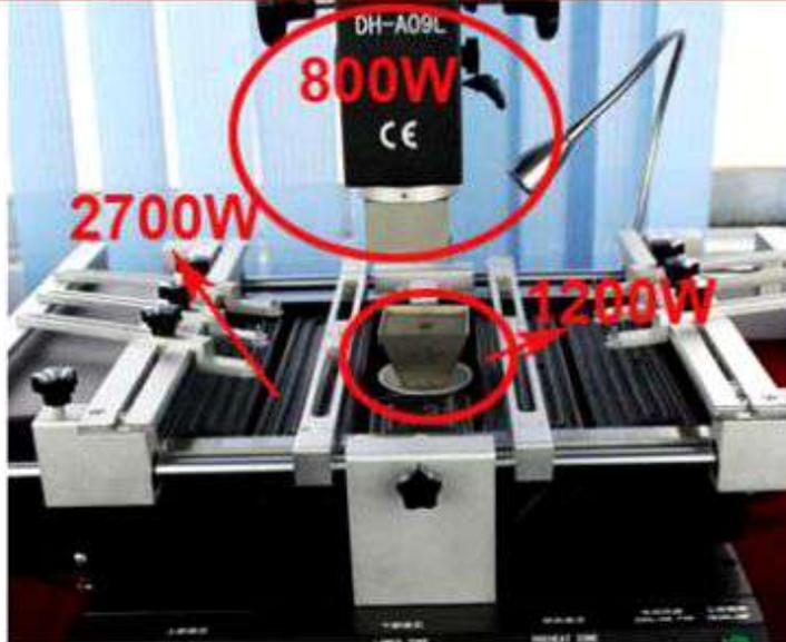
4. Nozzles with reflow, when the heating is over high, the cross flow air can turn automatic to help cooling the PCB board.
