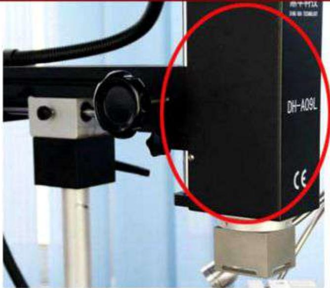
2. the upper heater can be moved up/down front/back, rotate freely
