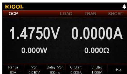
Figure 2-30 Main Interface of OCP Test Function
