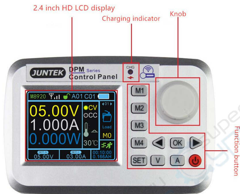
Figure 1-1 Description of the wireless control panel structure
