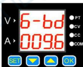
Short press **SET** to enter the baud rates selection interface, a total of 7 groups of baud rate, the unit is kbps, change the baud rates by pressing **▲** and **▼**, and then press the **OK** button, the setting is successful.
