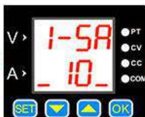
Long press **SET** to enter the voltage and current upper and lower limit save interface, change the sub-option by pressing **▲** and **▼**, 10 means the current voltage and current value is set to the upper limit, 11 means to set the lower limit, 12 means to cancel the upper and lower limit. Press **OK** and the setting is successful.
