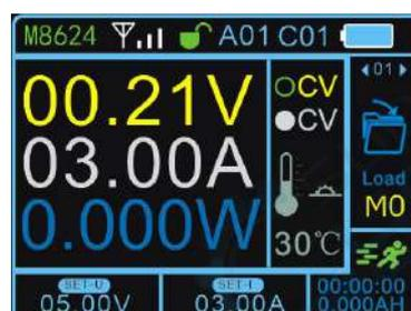
When the load current reaches the set current, the output is the set current, the constant current is output, and the CC light is on.
