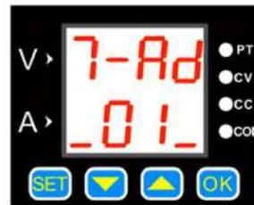
Short press **SET** to enter the local address selection interface, there are 99 groups of 01-99 communication address, change the communication address by pressing **▲** and **▼**, and then press the **OK** and the setting is successful.
