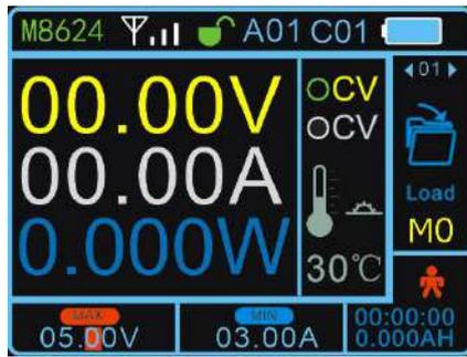
When the adjustment voltage and current reach the upper limit, it is displayed as MAX.
