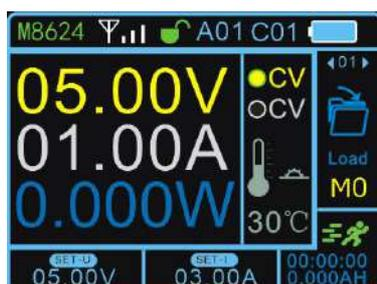
When the constant voltage output is 5V, 1A, and the load current is less than the set current, the output is constant voltage output, and the CV light is on.
