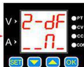
Short press **SET** to enter the factory reset interface, press **▲** and **▼** to change the sub-option, N means "no", Y means "yes", then press **OK**, the setting is
