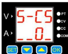
Short press **SET** to enter the communication protocol selection interface, and the sub-option is changed by pressing **▲** and **▼**. 0 means "simple communication protocol", 1 means "MODBUS-RTU communication protocol", then press **OK** button, the setting is successful.
