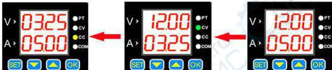
As the load current reaches the set current, the output is the set current, constant current output, CC light is on.
