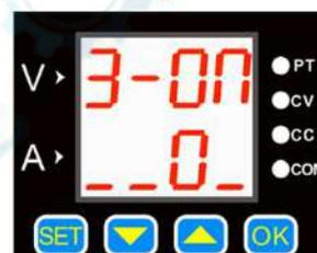
Short press **SET** to enter the power-on default output status interface, change the sub-option by pressing **▲** and **▼**, 0 means "off", 1 means "on", then press **OK**, the setting is
