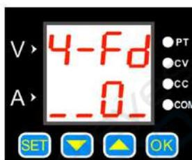
Short press **SET** to enter the fast response interface, and the sub-option is changed by pressing **▲** and **▼**. 0 means "slow", 1 means "fast", then press **OK**, the setting is successful.
