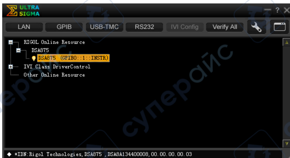
Figure 3-8 View the GPIB Resource
