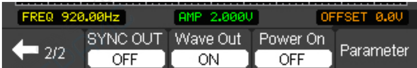
Figure 5-15 The Waveform Generator Waveform Window
