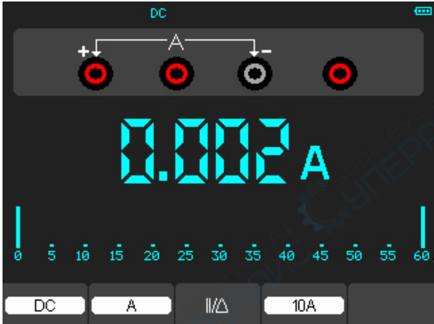
Figure 4-9 DC Current Measurement for 10A
