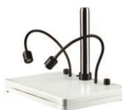
B3LS Pole Stand Vertical Post:240mm Dia.32mm Input Power:110v~240v, Double Gooseneck LED Illumination with an independent control Base Size:380x260x40mm Using with A1 Focusing Mount
