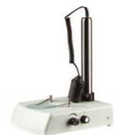
B2 Pole Stand Vertical Post:240mm Dia.32mm Top Halogen:12v/15w Bottom Halogen:12v/15w/ Fluorescent:7w Top and Bottom LED Illumination with an independent control Using with A1 Focusing Mount Base Size:200x255x60mm, with Φ95mm B/W Plastic Plate and Glass Plate and Paired Clips
