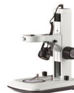
B9L Track Stand Vertical Height:300mm Focusing Distance:106mm Mounting Size:Φ76mm Input Power:110v~240v Top and Bottom LED Illumination with an independent control Base Size:205x275x40mm, with Φ95mm B/W Plastic & Perspex Plate and Paired Clips
