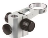
A1 Focusing Mount ID.32mm for Pole ID.76mm for Microscope Body Dist. Centre-to-centre:155mm The Vertical W.D.:50mm
