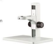
B2 Pole Stand Vertical Post:240mm Dia.32mm Top Halogen:12v/15w Bottom Halogen:12v/15w/ Fluorescent:7w Top and Bottom LED Illumination with an independent control Using with A1 Focusing Mount Base Size:200x255x60mm, with Φ95mm B/W Plastic Plate and Glass Plate and Paired Clips
