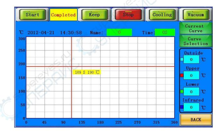
Click the button of "current curve", enter "START" to operate the heating lines we need. They are separately target temperature, onstant temperature time, and the speed of heating ( the speed of heating with C/SEC calculation).
