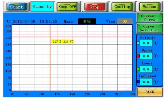
Three-zone tempertures can be set 6 levels of variable and constant temperature controls. If need, you can change the related parameters, but it's not saved, just can heat it with this line. If saveing is necessary, please refer to relative information of ingredient setting! If the temperature curve doesn't meet to the needed welding temperature; please press the return
