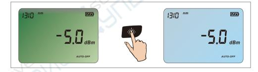
6 Measuring the optical power or loss. (Operation of power meter)
