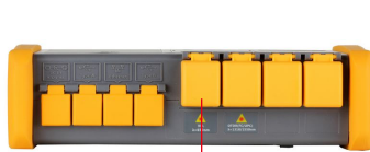
VFL launching port
