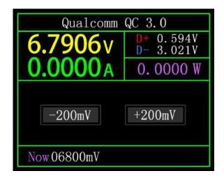
In QC3.0 trigger mode, Use the left and right keys to decrease/increase the trigger voltage, Click BACK to return. Press the left/right keys to quickly decrease/increase the voltage.
