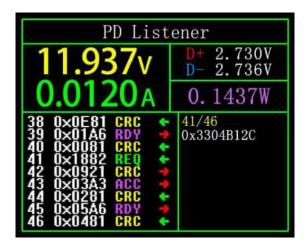
Click the middle button, Can switch to the page of "View detailed communication process", As shown above. Left column, You can select the message to be viewed by left/key, Such as:
