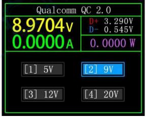
In QC2.0 trigger mode, use the left and right keys to select the trigger voltage, and click BACK to return.
