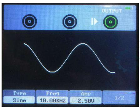
7. The waveform observed by an oscilloscope is as follows:
