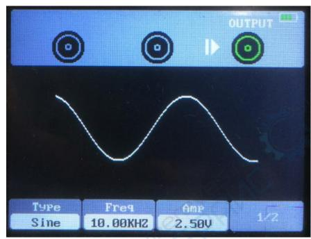
6. Press D button, the backlight of the button turns green, i.e. output sine waveform.
