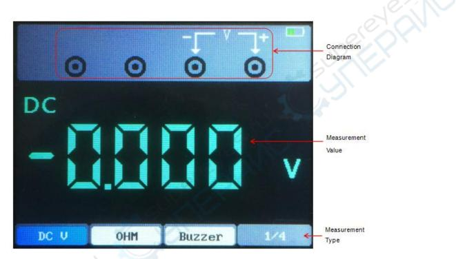
The measuring types include DC voltage (V, mV), AC voltage, DC current (A, mA), AC current (A, mA), resistance, capacitance, diode, and on-off test.
