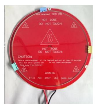
**Aluminium:** stick the thermistor to the back side of PCB heated bed by Kapton tape or similar.
