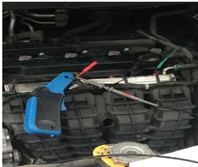
Pic-3 use of current clamp
