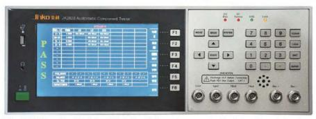
JK2828 high precision LCR Meter is a kind of multifunctional element parameters for the various electronic components inspection tester. With 7 inches 800 x480 color TFT LCD display, High speed and stability and more than 20 Hz = 1MHz frequency point and the accuracy of 0.05%, JK2828 is used for incoming inspection of components, quality of product line and goods inspection and laboratory measurement requirements etc.
