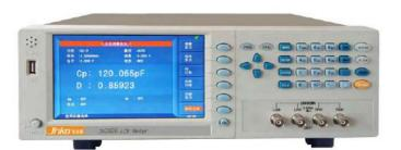
JK2826 high precision digital bridge is a kind of multifunctional component parameter tester for testing various electronic components. Using 7 inch 800x480 color TFT LCD. High speed, stable. 20Hz-5MHz multi frequency points and 0.05% accuracy can meet the require-ments of production line quality control, incoming inspection and laboratory measurements.
