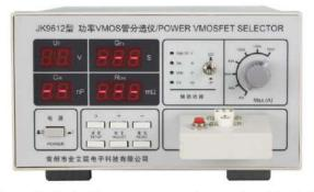
JK9612 Power VMOSFET selector is mainly used in the batch measurement and screening of the field effect transistor or IGBT in the small and medium-sized electronic products enterprises.
