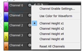
Click "Channel Enable Settings" in the menu, you could enable or close the appropriate channel in the Settings box.
