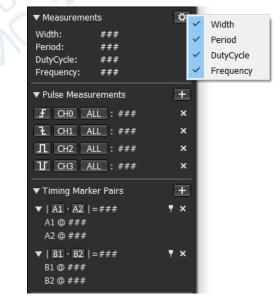
After some items have been selected, move the mouse inside the waveform window, the measurement results of where the mouse stays would display in the measurement window.
