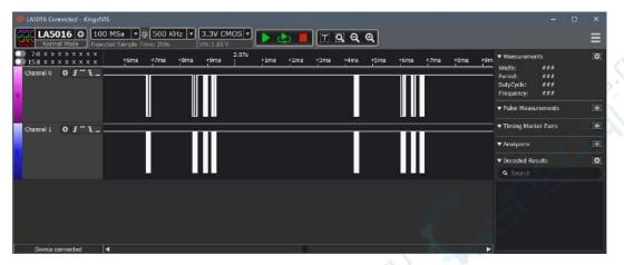
From this figure, we can see the coordinate values of the time axis are too large, and the effective waveform is within a very short period. You can click the left button of the mouse to zoom in the waveform; while the right button would zoom it out. And you can get these done with the mouse wheel too. After the waveform is zoomed up, you could see:
