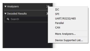
Click the "More Analyzers", and all the supported analyzers will be listed, as shown in the figure below.
