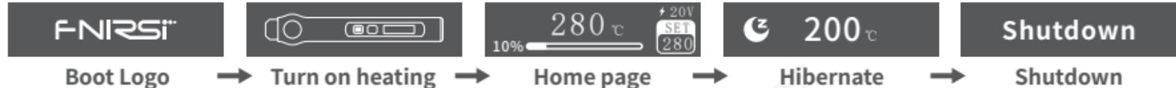
The working process of HS-01 intelligent soldering iron is shown in the figure above. After power-on, the logo is displayed. Short press the corresponding flashing physical button once to heat up. When the child lock mode is turned on, short press the corresponding physical button three times to heat. Entering the main interface, you can choose between 3 main working states of the soldering iron:
