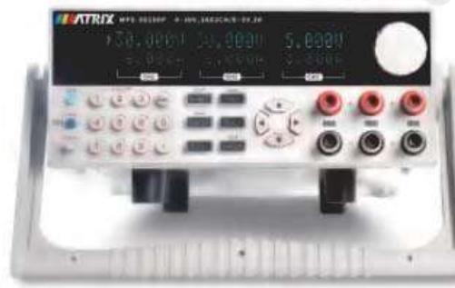
Tri-channel programmable DC power supply is with high resolution, high precision and high stability. Over-voltage and over-heat protection are available. Series and parallel operation are also provided. The resolution is 1 mV / 1 mA.
