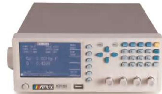
MCR5000 series is a multifunctional LCR precision meter used for testing various electronic components. Adopt 4.3-inch TFT LCD display, simple display, elegant layout. It is a high speed, wide band, 5 bit test resolution impedance measuring instrument with 40hz-200khz multiple frequency points and 0.1% accuracy, which can meet the requirements of component parameter detection in various occasions. Is a high - quality cost-effective tester
