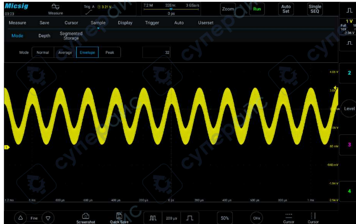
Figure 11-8 Signal in Envelope Sampling Mode (32)
