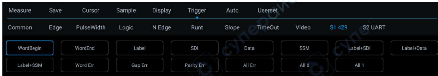
Figure 12-27 ARINC429 Trigger Mode Configuration Menu
