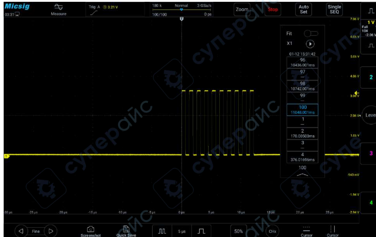
Figure 11-12 Segmented storage single frame viewing
