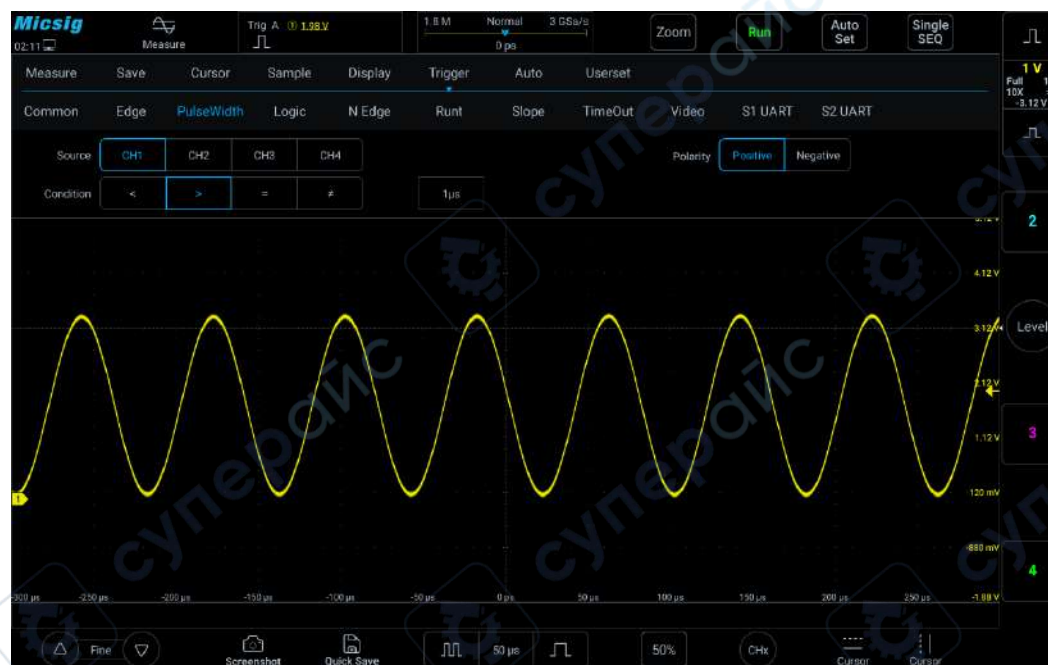
Figure 6-14 Pulse Width Trigger Setting Menu
