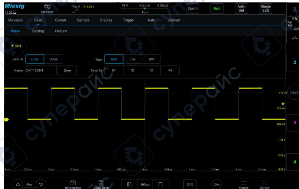
Figure 8-5 Save CH1 Reference Waveform Interface
