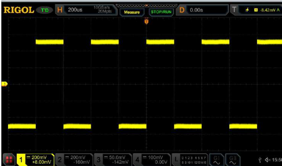
Figure 4-2 Waveforms before Averaging
