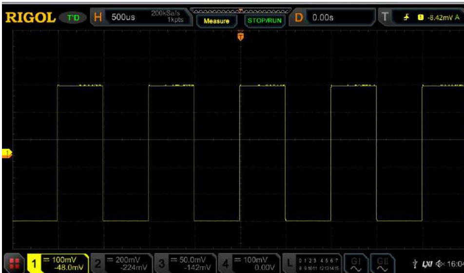
Figure 4-3 Waveforms after 128 Times of Averaging
