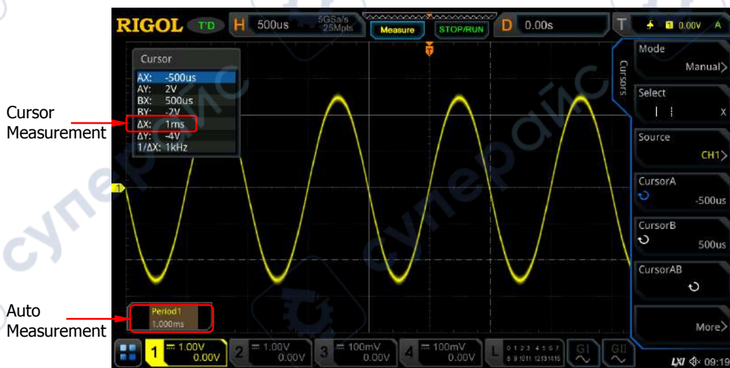
Figure 6-3 Manual Cursor Measurement Example
