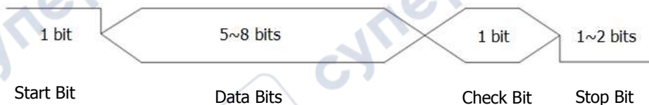
Figure 5-13 Schematic Diagram of RS232 Protocol
