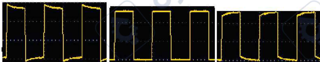
Overcompensated Compensated correctly Under compensated
