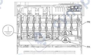
**NOTE:** Tightening torque of the M8 screws is 11.8 N.m (104.44 lbf.in) The width of the ring terminal should be 26 mm (1.02 in) or less.
