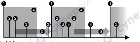
The figure below shows the periodic transmission of SYNC messages and synchronous and asynchronous PDOs, relative to the SYNC window:
