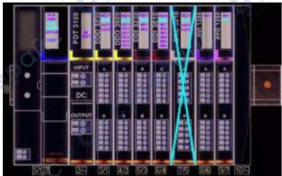
For example, when you physically construct the above configuration, you would build the island without the DRC-3210 and its base.
