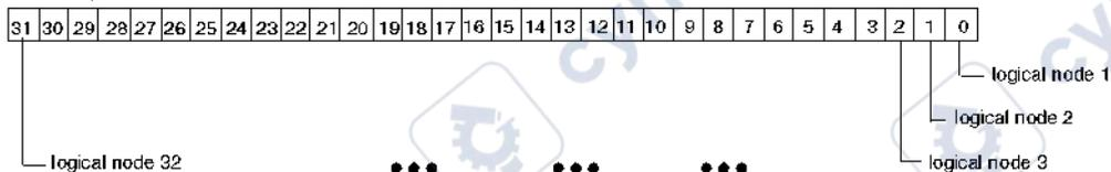
In the VPCR object, the bit pattern in subindex 1 represents the actual configuration being used by the island bus. When the fieldbus master makes a reconfiguration request, it should check this subindex in the VPCR object. After the reconfiguration request is successfully processed, the value in VPCR subindex 1 should be the same as the value in VPCW subindex 1.
