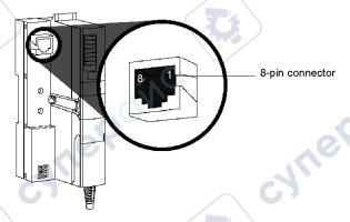
The RJ-45 connector is an 8-pin female connector. The pins connect horizontally along the top. Pin 8 has the leftmost position, and pin 1 is the rightmost. The connector pin-out is described in this table:
