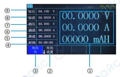
The Battery (battery) function simulates a charger to test the battery.
