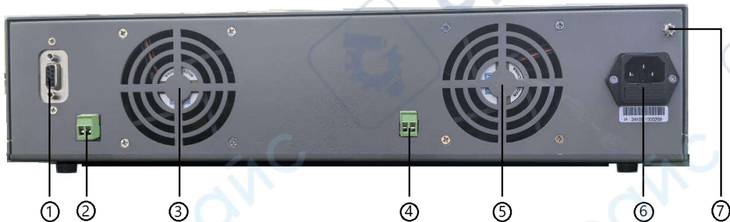
MTP-200 series programmable DC power supply back panel
