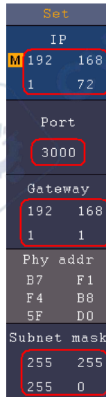
Figure 6-7 Set the network parameters of the oscilloscope
