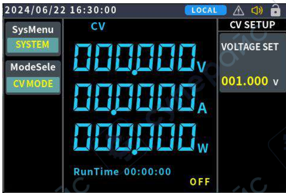
Figure 4.3.2-2 CV mode operation interface
