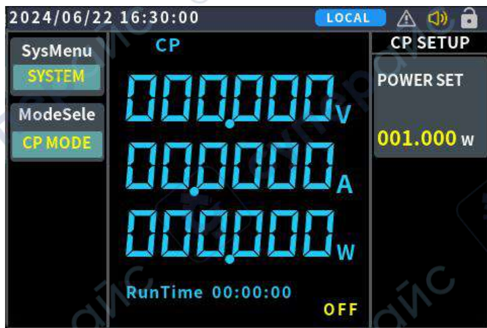
Figure 4.3.4-2 CP mode operation interface
