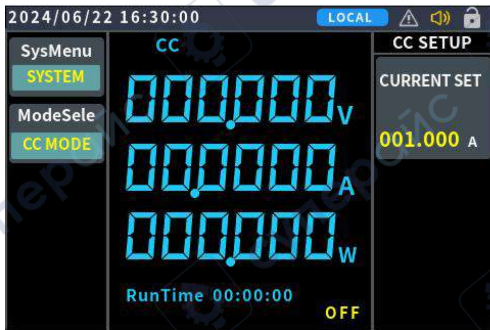
Figure 4.3.1-2 CC mode operation interface
