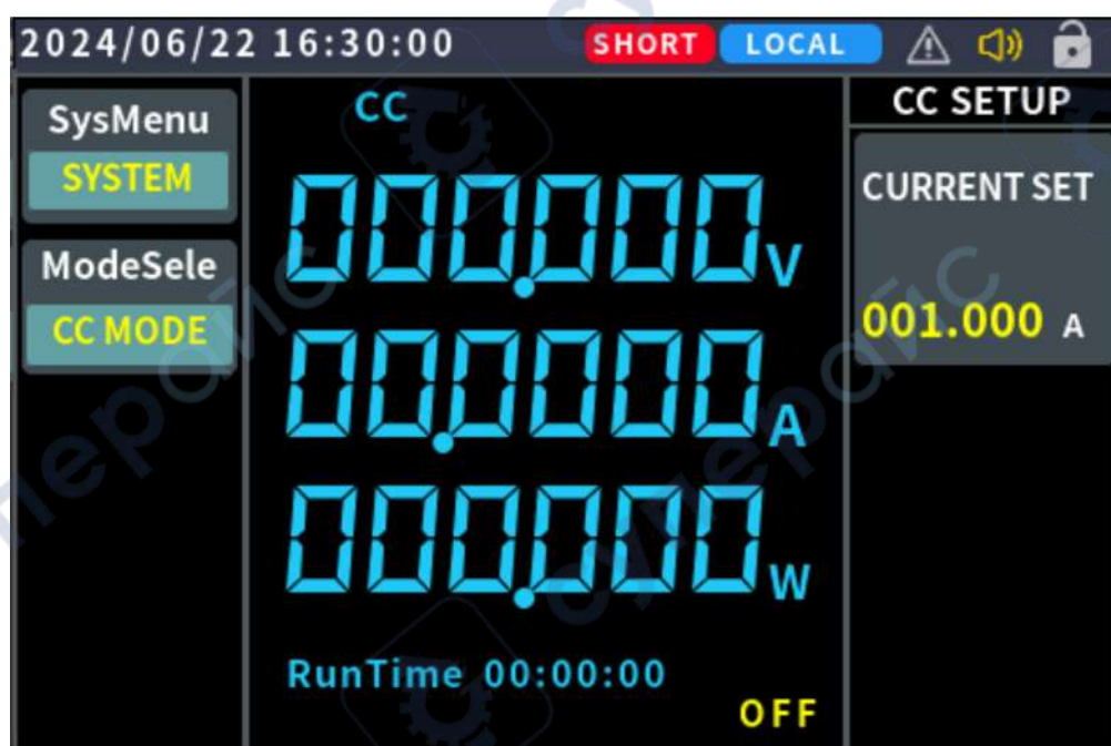
Figure 4.6-1 Short circuit simulation interface
