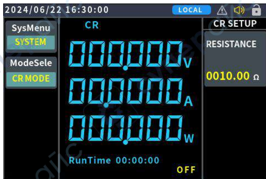
Figure 4.3.3-2 CR mode operation interface
