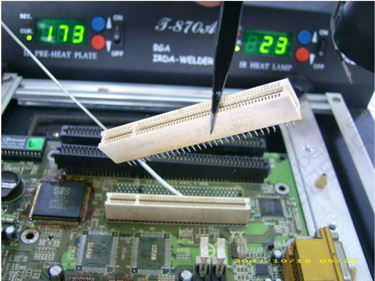
Removal of GAP slot
