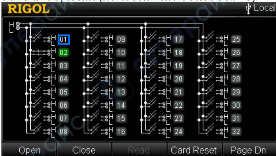
Figure 2-18 MC3132 Control Interface (Bank Joined)
