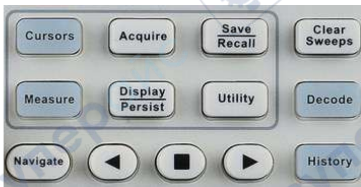
4-channel scope common function panel
