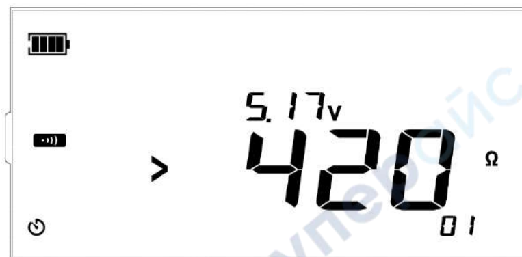
Figure 13.19 Low resistance exceeds the range
