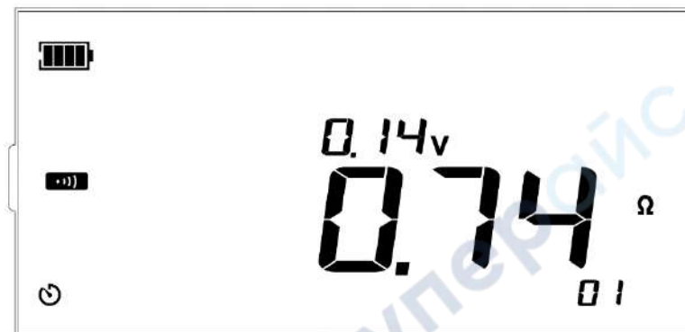
Figure 13.16 Test leads are shorted
