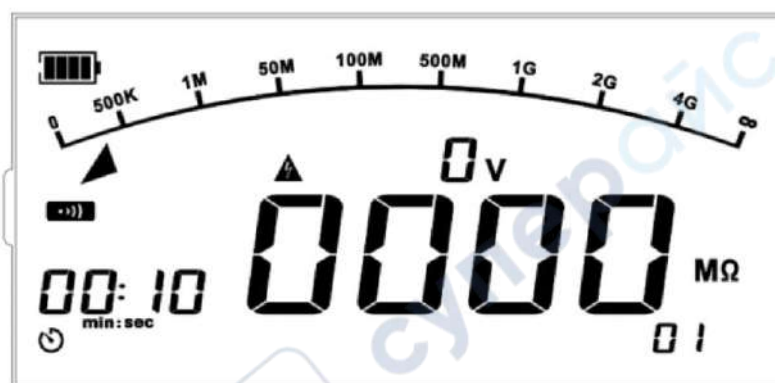
Figure 11.4 Test lead shorted
