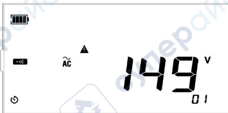
Figure 13.13 150VAC voltage measurement
