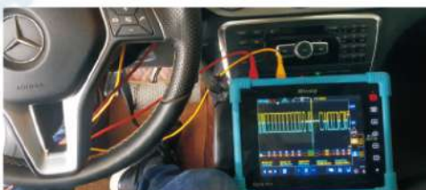
Power CAN bus communication
