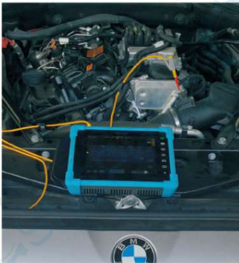
BMW Air flow meter test
