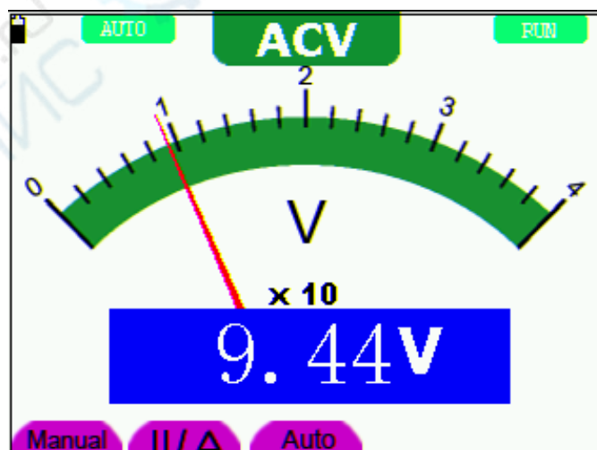
Figure 26: AC Voltage Measurement
