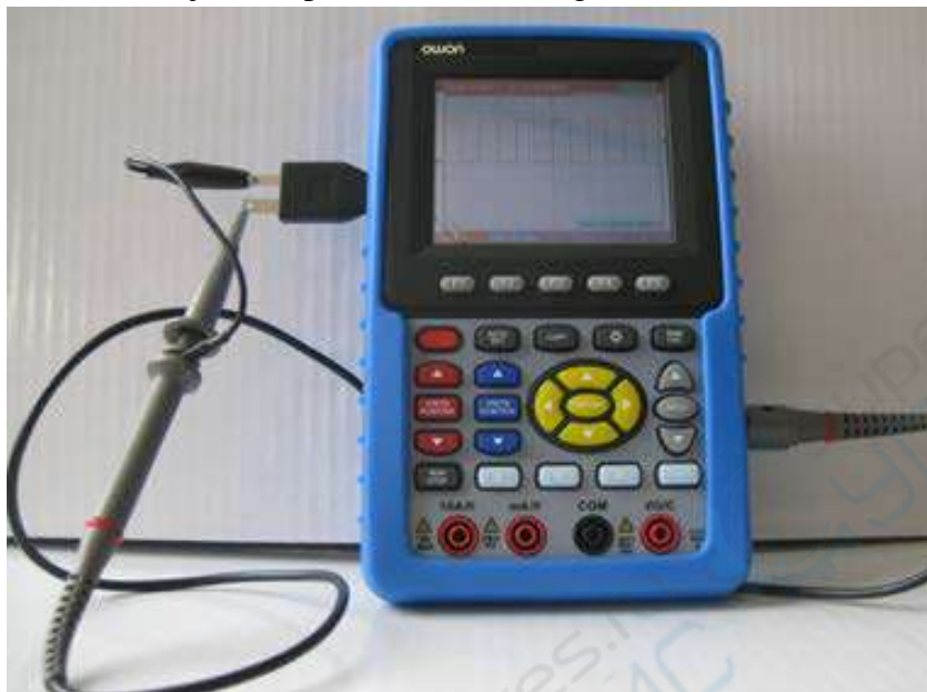
Fig.3. The connection of Square-wave test signal
