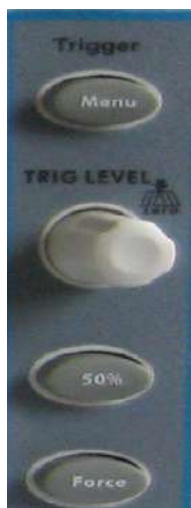
Figure 4-14 Trigger Control Zone
